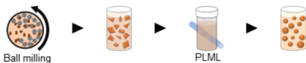
Figure 1. Schematic of preparation procedure of GaP NPs.
