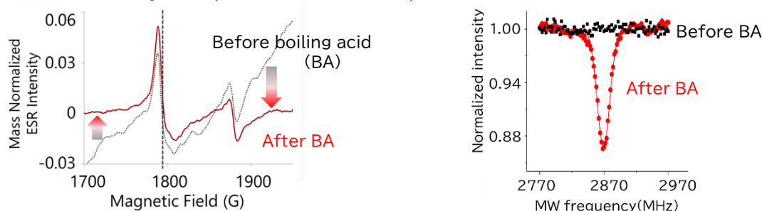
Fig.1 X-band ESR spectra of DNDs before/after boiling acid. Fig.2 CW-ODMR spectra of DNDs before/after boiling acid.
