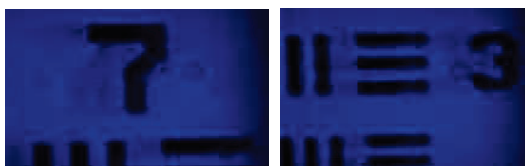
Figure 1: Laboratory calibration of microscopic unit with USAF 1951 resolution chart
