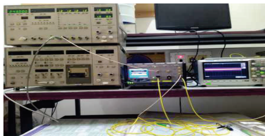
Fig. 2: Experimental setup for optical generation of PAM-4 signal.
